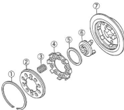
1. Retainer 5. Spacer 2. Spring Holder 6. Damper Cam 3. Damper Spring 7. Inner Hub 4. Spring Holder
